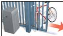
entrapment prevention system reverses gate on contact
